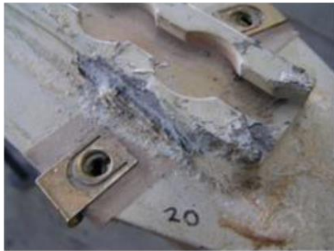
Fig. 3. A corroded seat track. Source: Lufthansa Technik, Laboratory Services
