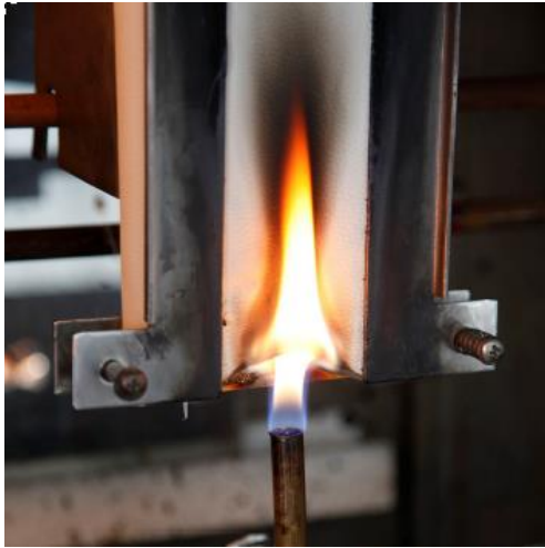
Figs. 7 & 8. Flammability testing with a Bunsen burner. Source: Lufthansa Technik, Laboratory Services
