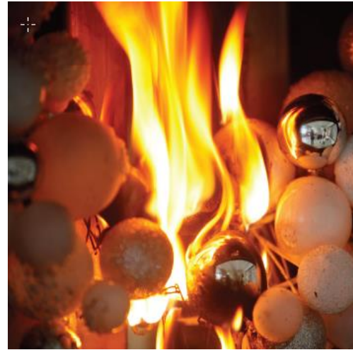
Figs. 7 & 8. Flammability testing with a Bunsen burner. Source: Lufthansa Technik, Laboratory Services
