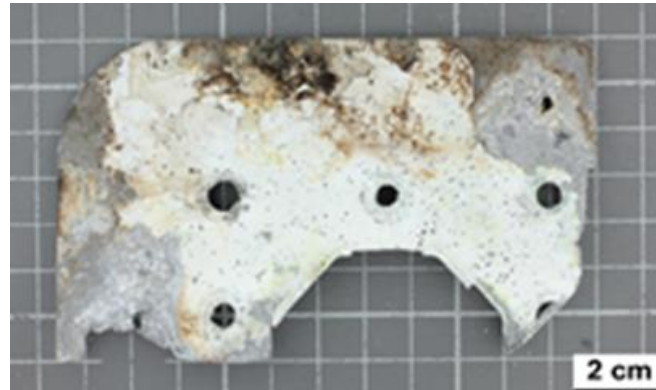
Fig. 2. An extremely corroded lavatory floor fitting. Source: Lufthansa Technik, Laboratory Services
