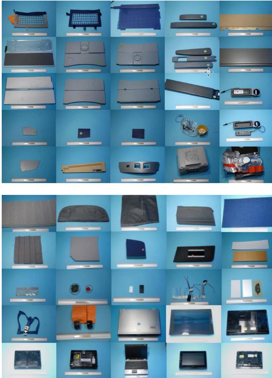
Figs. 4 & 5. Materials from the cabin interior used to test disinfectants. Source: Lufthansa Technik, Laboratory Services
